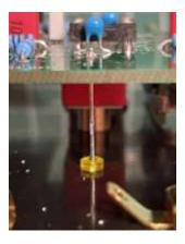
• Mounting the potentiometer. This will not fit exactly, because the original potentiometer is no longer available. A little improvisation is in order here.
