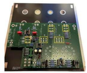
• Pay attention to the selector switches. There are numbers on the circuit board where the selector switches should be, and they should correspond to the numbers on the white bottom of the switch. See photo below.
