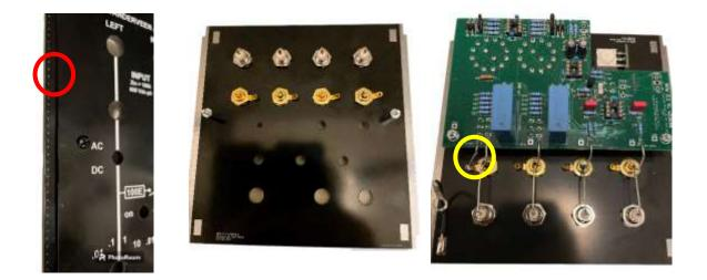
• Don't forget the LED. The LED must be placed before the PCB is soldered to the connectors. The square solder island for the LED on the PCB is the negative (cathode) side. There should be the short leg of the LED. And if not, try using a multimeter in diode mode. Determine the position of the LED in the work.
