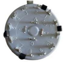
• The two selector switches have a locking ring supplied. These must be adjusted to the number (4) of positions required. First, turn the axis of the switch all the way to the left. Assemble the ring with the tooth in hole 4 (as shown in the photo on the right). It should now only switch 4 positions instead of 6 positions.
