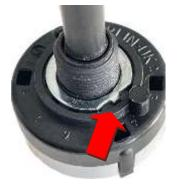
The connections of the BNC and RCA connectors can simply be made with bare wire. This doesn't have to be shielded either. The connectors are **not mounted in isolation** on the front panel. As a result, you only have to connect the ground to the circuit board in one place. See yellow circle in the photo. With this, the front panel is also connected to ground.
