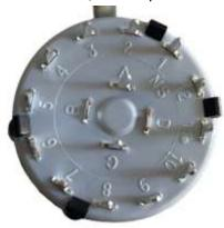
• The two selector switches have a locking ring supplied. These must be adjusted to the number (4) of positions required. First, turn the axis of the switch all the way to the left. Assemble the ring with the tooth in hole 4 (as shown in the photo on the right). It should now only switch 4 positions instead of 6 positions.
