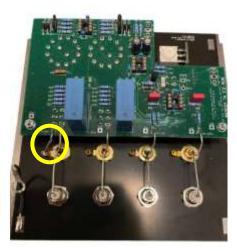
• Don't forget the LED. The LED must be placed before the PCB is soldered to the connectors. The square solder island for the LED on the PCB is the negative (cathode) side. There should be the short leg of the LED. And if not, try using a multimeter in diode mode. Determine the position of the LED in the work.
