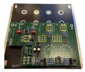
• Pay attention to the selector switches. There are numbers on the circuit board where the selector switches should be, and they should correspond to the numbers on the white bottom of the switch. See photo below.
