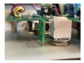
Due to the neck length of the toggle switches, the rotary switches may need to be fitted with a number of shims. These are not included in the BOM. You can use the black or red rings of the RCA connectors. You don't need it. Just drill out to 10mm. Adjust the rotary switches so that the neck of the toggle switches is flush with the top of the faceplate. See photo below. Finally, mount the supplied nuts of the selector switches and the volume knob on the top of the front panel.
